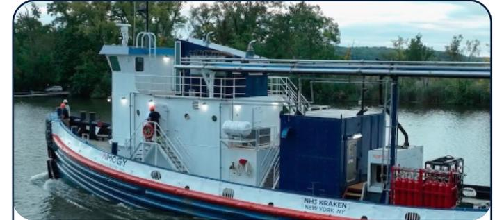
Amogy successfully **launched** the first carbon-free, ammonia powered maritime vessel, a tugboat **named NH<sub>3</sub> Kraken**. Amogy's ammonia cracking technology **converts** liquid ammonia (NH<sub>3</sub>) into its base elements of hydrogen and nitrogen, and then funnels the hydrogen into a fuel cell. The system is designed for vessels as small as a tugboat and as large as a containership and could also work in other heavy industries.
