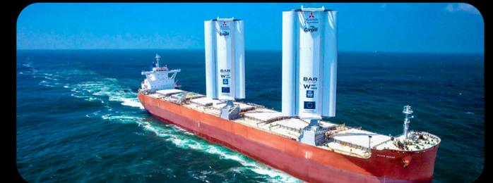
Mitsubishi's *Pyxis Ocean* [set sail](#) on its maiden voyage powered by WindWings, an advanced wind propulsion system. The *Pyxis Ocean* is retrofitted with two 37.5m-tall sails, with each wing saving 1.5 tons of fuel, or 4.65 tons of CO<sub>2</sub> emissions, per day.
